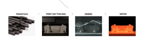
Given the proximity of the metal injection molding process and materials to the Studio System technology, the resulting metallurgy of Studio System parts is similar to metal injection molded parts.
