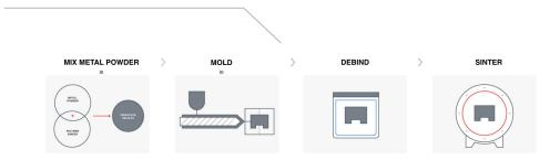
With BMD, the Studio System follows a similar process and utilizes the well-studied materials of in MIM. The Studio System media is a mixture of metal powder and Desktop Metal's proprietary binder in rod form. The bound metal rods are heated and extruded onto the build plate, shaping a part layer-by-layer.
